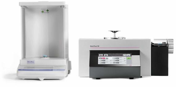
MultiTest 50 tablet hardness tester with integrated thickness gauge and connected analytical balance
