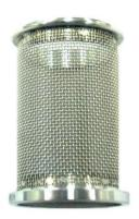
**USP Tolerances** Dimensions: Basket rim O.D. Ø 25.0 mm  $\pm 3.0$ mm Height 37.0 mm  $\pm 3.0$ mm Wire Ø 0.25 mm  $0.22 - 0.31 \, \text{mm}$ Wire openings 0.4 mm 0.36 - 0.44 mm Screen opening height 27.0 mm  $\pm 1.0$ mm Screen O.D. Ø 22.2 mm  $\pm 1.0$ mm Clear opening Ø 20.2 mm  $\pm 1.0$ mm
